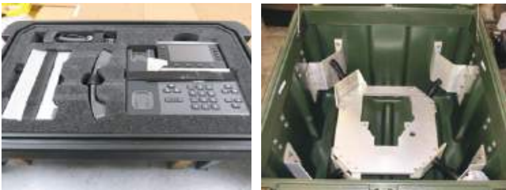
Fig. 3.2.5: Custom-made telecommunication equipment case
